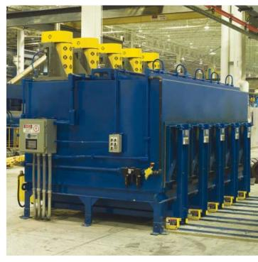
The Granco Clark multi-compartment die oven features individually heated drawers, minimizing heat loss and providing convenient die handling.
