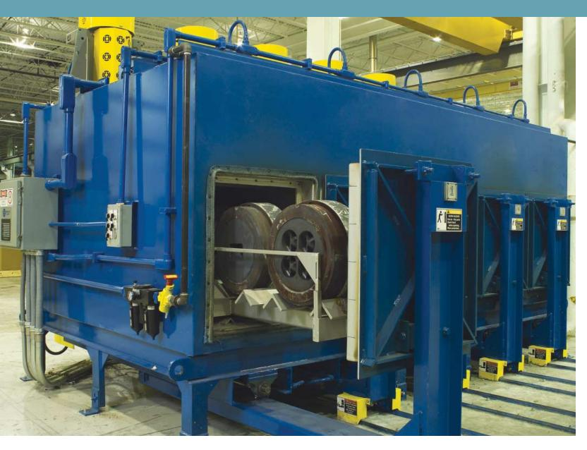
For the extrusion process to run smoothly, the right temperatures are key. And nowhere is this more important than at the press. Not only must the billet be heated to the correct temperature, the die must be as well. A die that isn't at the proper temperature when it's called for will slow your operation down and add stress to the press.
